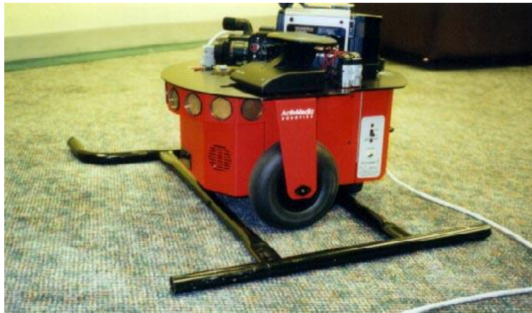
Figure 6 Immobilized by unseen obstruction
