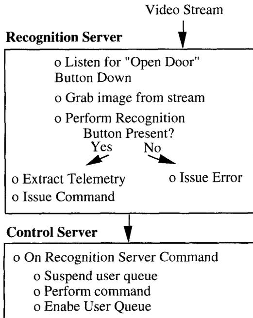
Figure 5 Recognition-Control Algorithm
