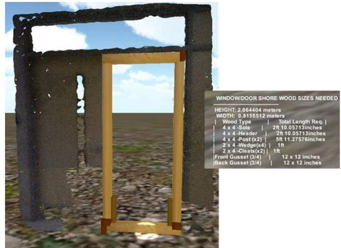
Fig. 1 The T-Spot and Window/Door shores constructed within DSR. The output materials are shown to the right.
