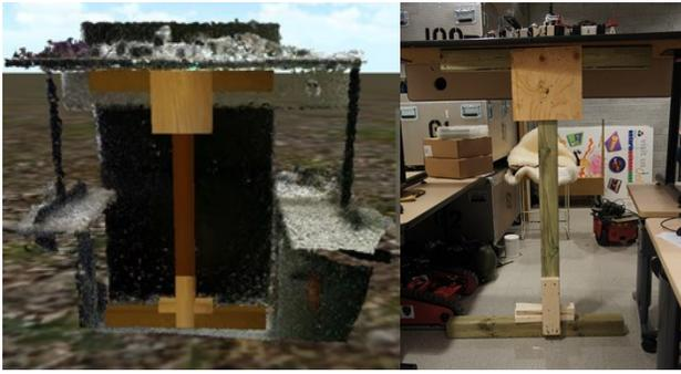
Fig. 7 Virtual shore created in DSR (left). Actual shore built from measurements supplied by DSR system (right).
