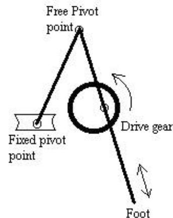
Figure 4 Middle Leg Drive Mechanism.
