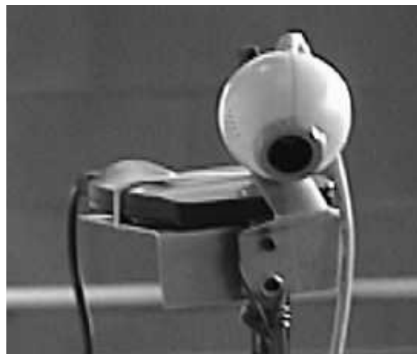
Figure 4 WiLan transceiver on CCD Camera Mast
