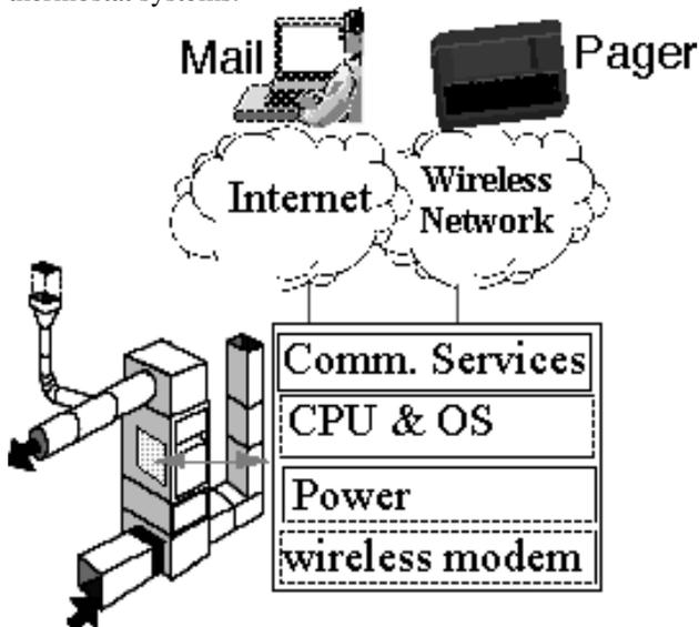
Figure 2 Internet Furnace Conceptual Architecture
