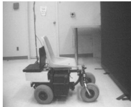
Fig. 2 Prototype Wheelchair
