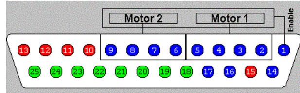
Fig. 5 Motors to parallel port connection
