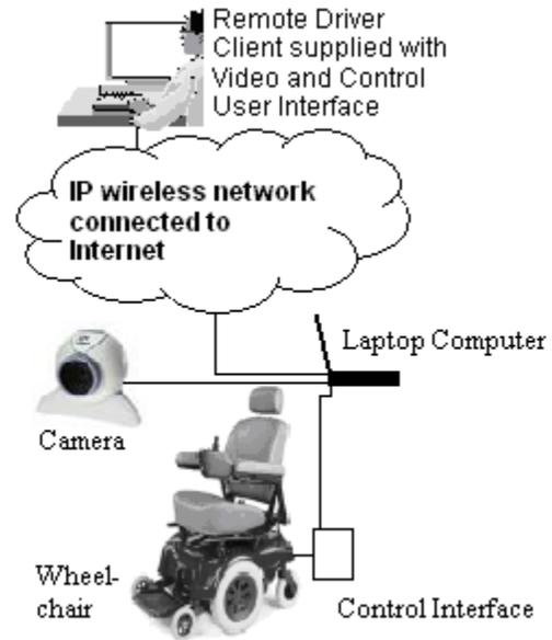
Fig. 1 System Conceptual Diagram
