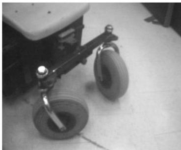
Fig. 10 Castor wheels on the front
