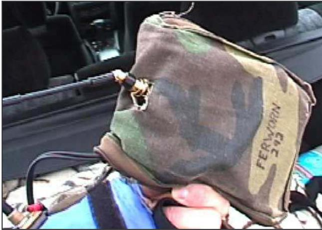
Fig. 6. CAT transceiver prototype as carried by handler
