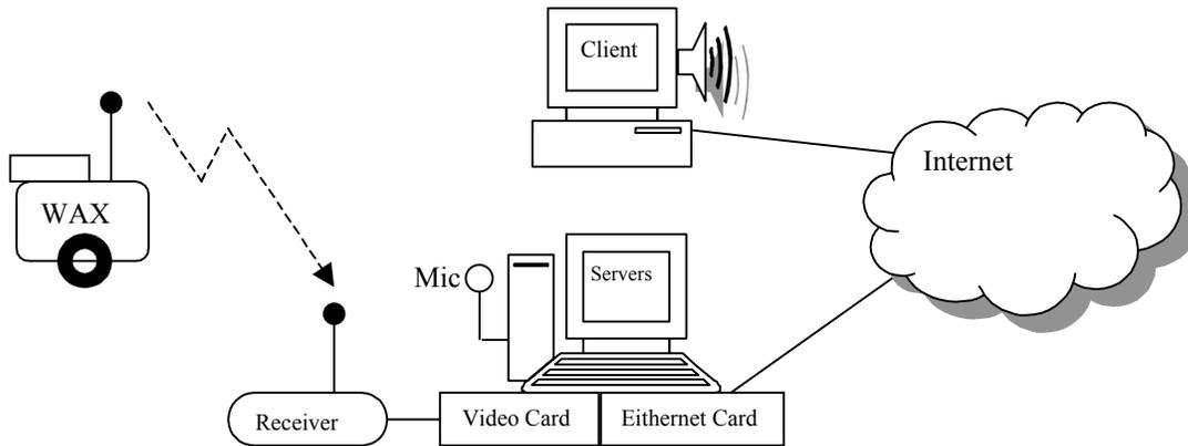
*Schematic of WAX's Configuration*
