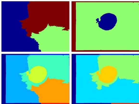
Fig. 2. Segmentation of colour image (top left), depth image (top right), overlaid segmentations (bottom left) and overlaid segmentations with merged segments (bottom right).
