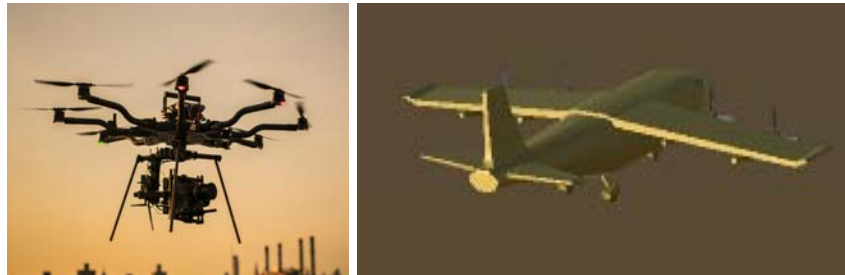
Fig. 7. Left: Freefly ATLA version 8, with 6 rotors [27], represented by the image on the right: a standard mini airplane model to fly to a location and deliver a payload.
