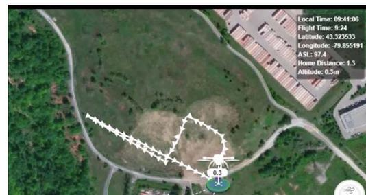
Fig. 2. Experiment 1: The complete route of the second attempt. Time to locate the test person was less than 7 minutes.
