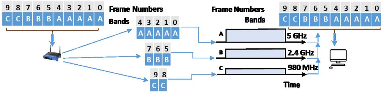
Fig. 1. A simplified model of the considered multi-band Wireless LAN
