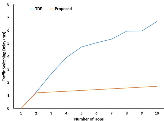
Fig. 5. Switching Delay with respected to number of hops.
