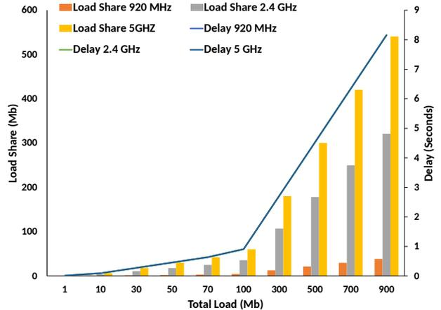
Fig. 3. Delay and Load Distribution Performance with respect to Incoming Load.
