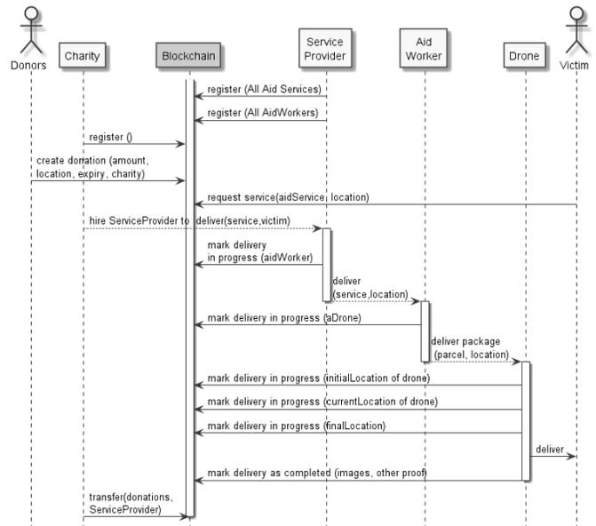
Fig. 4. The sequence of steps while delivering services with a drone
